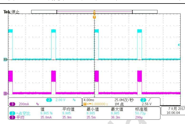
图 13, PWM 调光(100Hz/10%) (CH2:PWM CH3:Iout)
